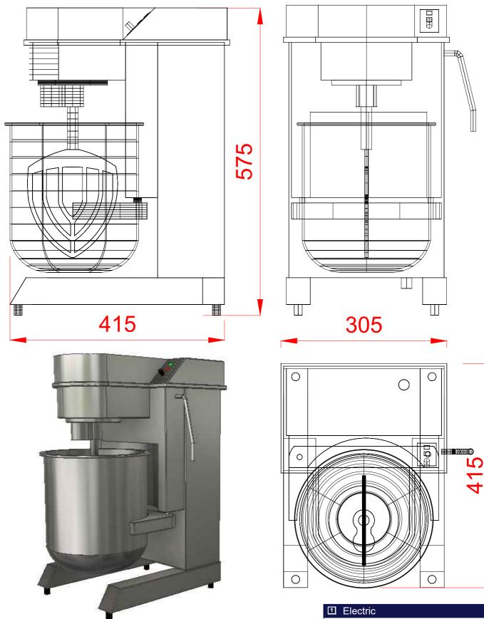
230/50/1 0.35kW 3.5amps MIXER COMES WITH 13amp PLUG FITTED WITH 13amp FUSE.
